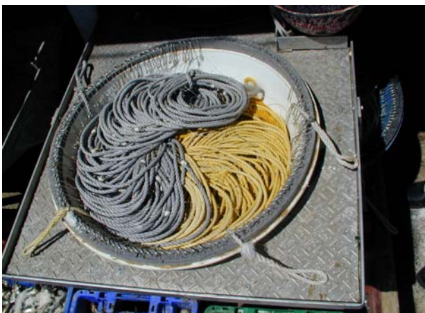
Figure 7. Standard hake longline pot as prepared prior to shooting of the line. Pots comprise normally of four lines of 25-30 hooks per line (source : CapFish)
